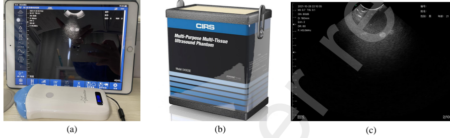
Figure 6: The equipment of our experiments. (a) is the handheld ultrasound equipment, (b) is the ultrasound phantom, (c) is an ultrasound image with 5MHz center frequency of the probe.
